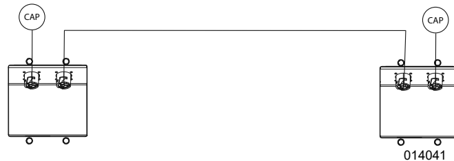
Figure 3-7. Two Units in Parallel
