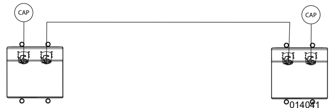
Figure 3-7. Two Units in Parallel
